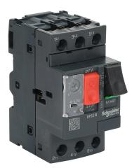
Schneider Electric Easy TeSys series manual motor protector, pushbutton, 6.3A, thermal overload, 4-6.3 adjustable, 78A instantaneous trip rating, 45mm frame.
