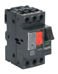
Schneider Electric Easy TeSys series manual motor protector, pushbutton, 2.5A, thermal overload, 1.6-2.5 adjustable, 33.5A instantaneous trip rating, 45mm frame.
