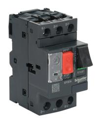
Schneider Electric Easy TeSys series manual motor protector, pushbutton, 1.6A, thermal overload, 1-1.6 adjustable, 22.5A instantaneous trip rating, 45mm frame.
