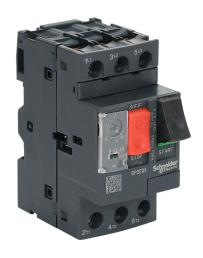
Schneider Electric Easy TeSys series manual motor protector, pushbutton, 1A, thermal overload, 0.63-1 adjustable, 13A instantaneous trip rating, 45mm frame.
