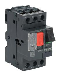
Schneider Electric Easy TeSys series manual motor protector, pushbutton, 0.63A, thermal overload, 0.40-0.63 adjustable, 8A instantaneous trip rating, 45mm frame.
