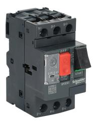
Schneider Electric Easy TeSys series manual motor protector, pushbutton, 0.4A, thermal overload, 0.25-0.40 adjustable, 5A instantaneous trip rating, 45mm frame.
