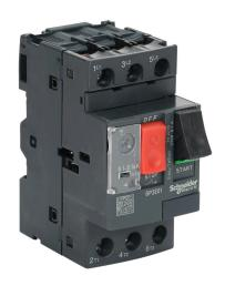
Schneider Electric Easy TeSys series manual motor protector, pushbutton, 0.16A, thermal overload, 0.1-0.16 adjustable, 1.5A instantaneous trip rating, 45mm frame.
