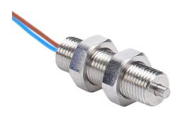
Metrol limit switch, vacuum, precision touch, 5mm diameter, threaded, 0.5mm pitch, 18.5mm length, 2mm radius head, stainless steel, 1.5mm plunger, 0.5N contact force, (1) N.C. contact(s), 1.6ft/0.5m cable length, core wire.
