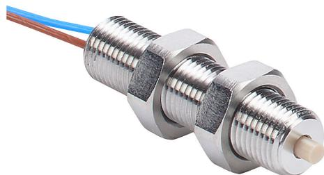
Metrol limit switch, vacuum, precision touch, 5mm diameter, threaded, 0.5mm pitch, 21.5mm length, 2mm radius head, stainless steel, 1.5mm plunger, 0.5N contact force, (1) N.O. contact(s), 1.6ft/0.5m cable length, core wire.
