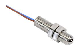
Metrol limit switch, vacuum, precision touch, 5mm diameter, threaded, 0.5mm pitch, 19mm length, 3mm head, ball plunger, 1N contact force, N.O. contact(s), 1.6ft/0.5m cable length, pigtail.
