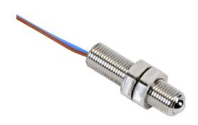
Metrol limit switch, vacuum, precision touch, 5mm diameter, threaded, 0.5mm pitch, 19mm length, 3mm head, stainless steel, ball plunger, 1N contact force, (1) N.O. contact(s), 1.6ft/0.5m cable length, pigtail.
