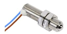
Metrol limit switch, vacuum, precision touch, 5mm diameter, threaded, 0.5mm pitch, 19mm length, 3mm head, stainless steel, ball plunger, 1N contact force, (1) N.O. contact(s), 1.6ft/0.5m cable length, pigtail.
