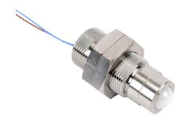
Metrol limit switch, vacuum, precision touch, 16mm diameter, threaded, 1mm pitch, 41mm length, 9.5mm head, 2mm plunger, 1.5N contact force, N.C. contact(s), 1.6ft/0.5m cable length, pigtail.
