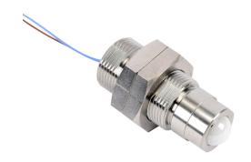
Metrol limit switch, vacuum, precision touch, 16mm diameter, threaded, 1mm pitch, 41mm length, 9.5mm head, stainless steel, 2mm plunger, 1.5N contact force, (1) N.C. contact(s), 1.6ft/0.5m cable length, pigtail.
