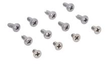
Integra rail screw kit, replacement. For use with Multi-Max series internal mounting rails. Includes (4) #10-32 x 0.38in stainless steel flat head screws and (8) #10-32 x 0.50in stainless steel pan head thread-cutting screws.
