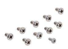
Integra mounting flange screw kit, replacement. For use with 24 x 24 x 10in Genesis series enclosures. Includes (10) 1/4-20 UNC x 0.050in stainless steel Phillips pan head screws and (1)  $\#10-32 \times 0.50$  in stainless steel pan head thread-cutting screw.
