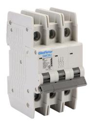
Gladiator miniature circuit breaker, 8A, 480Y / 277 VAC / 125 VDC, 3-pole, D curve, thermal magnetic, 10kA @ 480Y/277 VAC interrupting rating, 35mm DIN rail mount.
