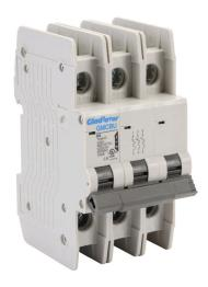
Gladiator miniature circuit breaker, 6A, 480Y / 277 VAC / 125 VDC, 3-pole, D curve, thermal magnetic, 10kA @ 480Y/277 VAC interrupting rating, 35mm DIN rail mount.
