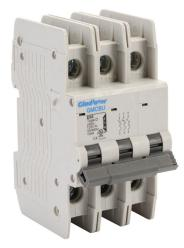
Gladiator miniature circuit breaker, 63A, 240 VAC / 125 VDC, 3-pole, D curve, thermal magnetic, 10kA @ 240 VAC interrupting rating, 35mm DIN rail mount.
