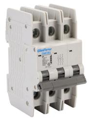
Gladiator miniature circuit breaker, 5A, 480Y / 277 VAC / 125 VDC, 3-pole, D curve, thermal magnetic, 10kA @ 480Y/277 VAC interrupting rating, 35mm DIN rail mount.
