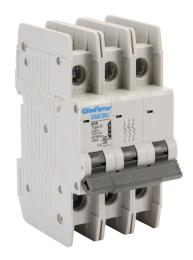
Gladiator miniature circuit breaker, 50A, 240 VAC / 125 VDC, 3-pole, D curve, thermal magnetic, 10kA @ 240 VAC interrupting rating, 35mm DIN rail mount.
