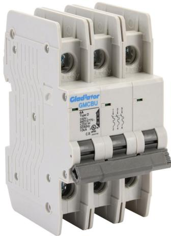
Gladiator miniature circuit breaker, 4A, 480Y / 277 VAC / 125 VDC, 3-pole, D curve, thermal magnetic, 10kA @ 480Y/277 VAC interrupting rating, 35mm DIN rail mount.
