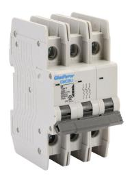
Gladiator miniature circuit breaker, 4A, 480Y / 277 VAC / 125 VDC, 3-pole, D curve, thermal magnetic, 10kA @ 480Y/277 VAC interrupting rating, 35mm DIN rail mount.
