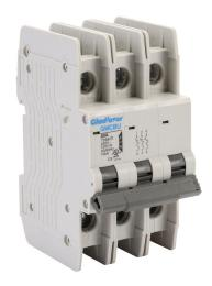
Gladiator miniature circuit breaker, 40A, 240 VAC / 125 VDC, 3-pole, D curve, thermal magnetic, 10kA @ 240 VAC interrupting rating, 35mm DIN rail mount.
