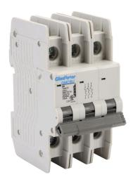
Gladiator miniature circuit breaker, 3A, 480Y / 277 VAC / 125 VDC, 3-pole, D curve, thermal magnetic, 10kA @ 480Y/277 VAC interrupting rating, 35mm DIN rail mount.
