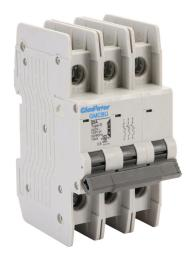
Gladiator miniature circuit breaker, 32A, 240 VAC / 125 VDC, 3-pole, D curve, thermal magnetic, 10kA @ 240 VAC interrupting rating, 35mm DIN rail mount.
