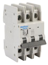
Gladiator miniature circuit breaker, 2A, 480Y / 277 VAC / 125 VDC, 3-pole, D curve, thermal magnetic, 10kA @ 480Y/277 VAC interrupting rating, 35mm DIN rail mount.
