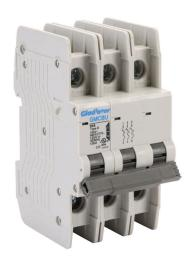
Gladiator miniature circuit breaker, 25A, 480Y / 277 VAC / 125 VDC, 3-pole, D curve, thermal magnetic, 10kA @ 480Y/277 VAC interrupting rating, 35mm DIN rail mount.
