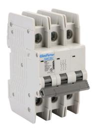
Gladiator miniature circuit breaker, 20A, 480Y / 277 VAC / 125 VDC, 3-pole, D curve, thermal magnetic, 10kA @ 480Y/277 VAC interrupting rating, 35mm DIN rail mount.
