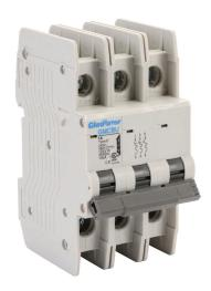
Gladiator miniature circuit breaker, 1A, 480Y / 277 VAC / 125 VDC, 3-pole, D curve, thermal magnetic, 10kA @ 480Y/277 VAC interrupting rating, 35mm DIN rail mount.
