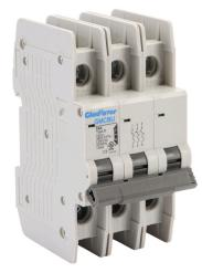
Gladiator miniature circuit breaker, 16A, 480Y / 277 VAC / 125 VDC, 3-pole, D curve, thermal magnetic, 10kA @ 480Y/277 VAC interrupting rating, 35mm DIN rail mount.
