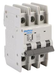
Gladiator miniature circuit breaker, 15A, 480Y / 277 VAC / 125 VDC, 3-pole, D curve, thermal magnetic, 10kA @ 480Y/277 VAC interrupting rating, 35mm DIN rail mount.
