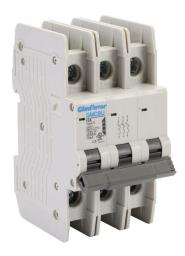
Gladiator miniature circuit breaker, 10A, 480Y / 277 VAC / 125 VDC, 3-pole, D curve, thermal magnetic, 10kA @ 480Y/277 VAC interrupting rating, 35mm DIN rail mount.
