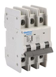
Gladiator miniature circuit breaker, 8A, 480Y / 277 VAC / 125 VDC, 3-pole, C curve, thermal magnetic, 10kA @ 480Y/277 VAC interrupting rating, 35mm DIN rail mount.
