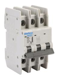
Gladiator miniature circuit breaker, 63A, 240 VAC / 125 VDC, 3-pole, C curve, thermal magnetic, 10kA @ 240 VAC interrupting rating, 35mm DIN rail mount.
