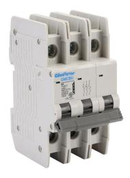
Gladiator miniature circuit breaker, 5A, 480Y / 277 VAC / 125 VDC, 3-pole, C curve, thermal magnetic, 10kA @ 480Y/277 VAC interrupting rating, 35mm DIN rail mount.
