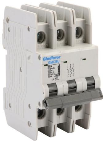
Gladiator miniature circuit breaker, 50A, 240 VAC / 125 VDC, 3-pole, C curve, thermal magnetic, 10kA @ 240 VAC interrupting rating, 35mm DIN rail mount.
