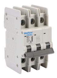
Gladiator miniature circuit breaker, 40A, 240 VAC / 125 VDC, 3-pole, C curve, thermal magnetic, 10kA @ 240 VAC interrupting rating, 35mm DIN rail mount.
