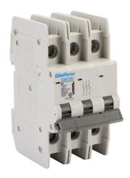
Gladiator miniature circuit breaker, 3A, 480Y / 277 VAC / 125 VDC, 3-pole, C curve, thermal magnetic, 10kA @ 480Y/277 VAC interrupting rating, 35mm DIN rail mount.
