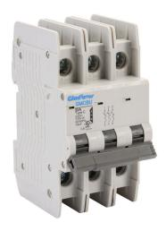
Gladiator miniature circuit breaker, 32A, 240 VAC / 125 VDC, 3-pole, C curve, thermal magnetic, 10kA @ 240 VAC interrupting rating, 35mm DIN rail mount.
