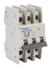
Gladiator miniature circuit breaker, 2A, 480Y / 277 VAC / 125 VDC, 3-pole, C curve, thermal magnetic, 10kA @ 480Y/277 VAC interrupting rating, 35mm DIN rail mount.
