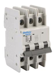
Gladiator miniature circuit breaker, 25A, 480Y / 277 VAC / 125 VDC, 3-pole, C curve, thermal magnetic, 10kA @ 480Y/277 VAC interrupting rating, 35mm DIN rail mount.
