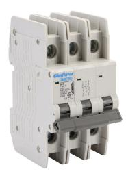
Gladiator miniature circuit breaker, 20A, 480Y / 277 VAC / 125 VDC, 3-pole, C curve, thermal magnetic, 10kA @ 480Y/277 VAC interrupting rating, 35mm DIN rail mount.
