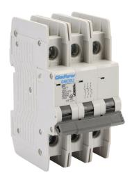
Gladiator miniature circuit breaker, 20A, 480Y / 277 VAC / 125 VDC, 3-pole, C curve, thermal magnetic, 10kA @ 480Y/277 VAC interrupting rating, 35mm DIN rail mount.
