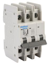
Gladiator miniature circuit breaker, 1A, 480Y / 277 VAC / 125 VDC, 3-pole, C curve, thermal magnetic, 10kA @ 480Y/277 VAC interrupting rating, 35mm DIN rail mount.
