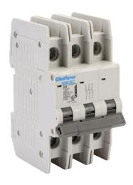
Gladiator miniature circuit breaker, 16A, 480Y / 277 VAC / 125 VDC, 3-pole, C curve, thermal magnetic, 10kA @ 480Y/277 VAC interrupting rating, 35mm DIN rail mount.
