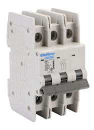
Gladiator miniature circuit breaker, 15A, 480Y / 277 VAC / 125 VDC, 3-pole, C curve, thermal magnetic, 10kA @ 480Y/277 VAC interrupting rating, 35mm DIN rail mount.
