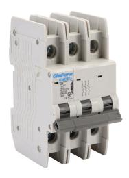
Gladiator miniature circuit breaker, 10A, 480Y / 277 VAC / 125 VDC, 3-pole, C curve, thermal magnetic, 10kA @ 480Y/277 VAC interrupting rating, 35mm DIN rail mount.
