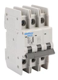
Gladiator miniature circuit breaker, 8A, 480Y / 277 VAC / 125 VDC, 3-pole, B curve, thermal magnetic, 10kA @ 480Y/277 VAC interrupting rating, 35mm DIN rail mount.
