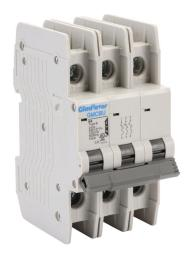
Gladiator miniature circuit breaker, 6A, 480Y / 277 VAC / 125 VDC, 3-pole, B curve, thermal magnetic, 10kA @ 480Y/277 VAC interrupting rating, 35mm DIN rail mount.
