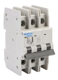
Gladiator miniature circuit breaker, 6A, 480Y / 277 VAC / 125 VDC, 3-pole, B curve, thermal magnetic, 10kA @ 480Y/277 VAC interrupting rating, 35mm DIN rail mount.
