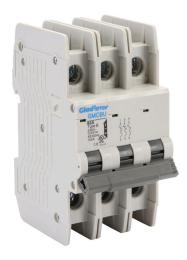
Gladiator miniature circuit breaker, 63A, 240 VAC / 125 VDC, 3-pole, B curve, thermal magnetic, 10kA @ 240 VAC interrupting rating, 35mm DIN rail mount.
