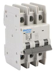
Gladiator miniature circuit breaker, 5A, 480Y / 277 VAC / 125 VDC, 3-pole, B curve, thermal magnetic, 10kA @ 480Y/277 VAC interrupting rating, 35mm DIN rail mount.
