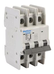
Gladiator miniature circuit breaker, 50A, 240 VAC / 125 VDC, 3-pole, B curve, thermal magnetic, 10kA @ 240 VAC interrupting rating, 35mm DIN rail mount.
