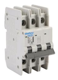
Gladiator miniature circuit breaker, 4A, 480Y / 277 VAC / 125 VDC, 3-pole, B curve, thermal magnetic, 10kA @ 480Y/277 VAC interrupting rating, 35mm DIN rail mount.
